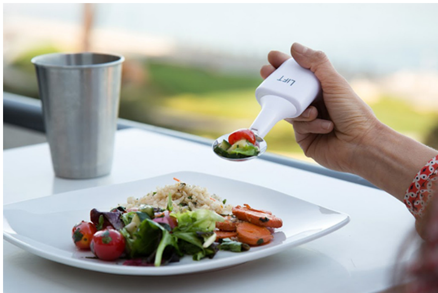
This spoon from Liftware can counteract hand tremors. Liftware
